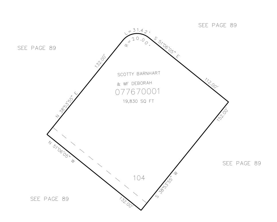
10' UTILITY & DRAINAGE EASEMENTS EACH SIDE OF PROPERTY LINES AS INDICATED BY DASHED LINES EXCEPT AS OTHERWISE SHOWN.
